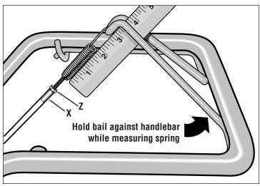
Fig. 2-7: Measure cable spring.
